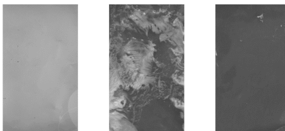
Figure 1. Photographs of the 2-layer laminate sample in different stages of dissolution: (a) pre-dissolution; (b) mid-dissolution; (c) post-dissolution.
