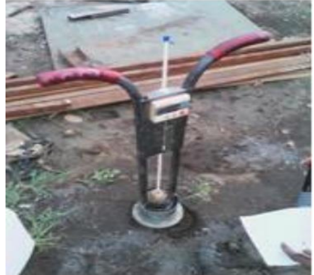
Fig 5. Turftec Double ring infiltrometer (Source: D Noorvy Khaerudin)
